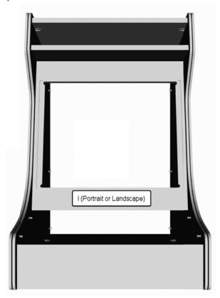
8. Install the H Panel, this is a good time to install buttons, joystick and wiring. Turn the unit around and use the stubby screwdriver to secure the camlocks.
