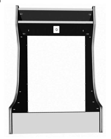
7. Choose the orientation for the monitor and install the I panel. You will need to lift the G panel as it will rotate on the camlocks, align the G panel to the I panel so that the camlocks engage the camlock studs on the G panel.
