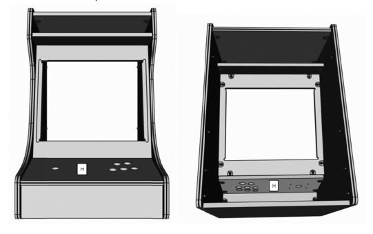
9. From the back of the unit install the E panel. This is a good time to install the electronic components.
